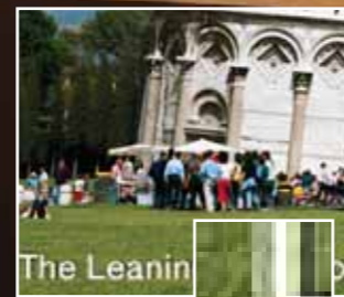
With MPEG Noise Reduction turned off, subtitles on screen appear blurry and difficult to read.
